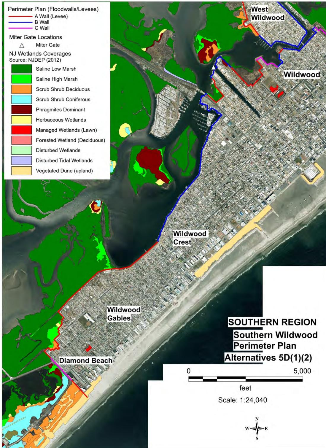
Figure 60: Perimeter Plan Overlay with Wetland Habitats along Wildwood (south) Alignment in Alternatives 5D(1)(2)
