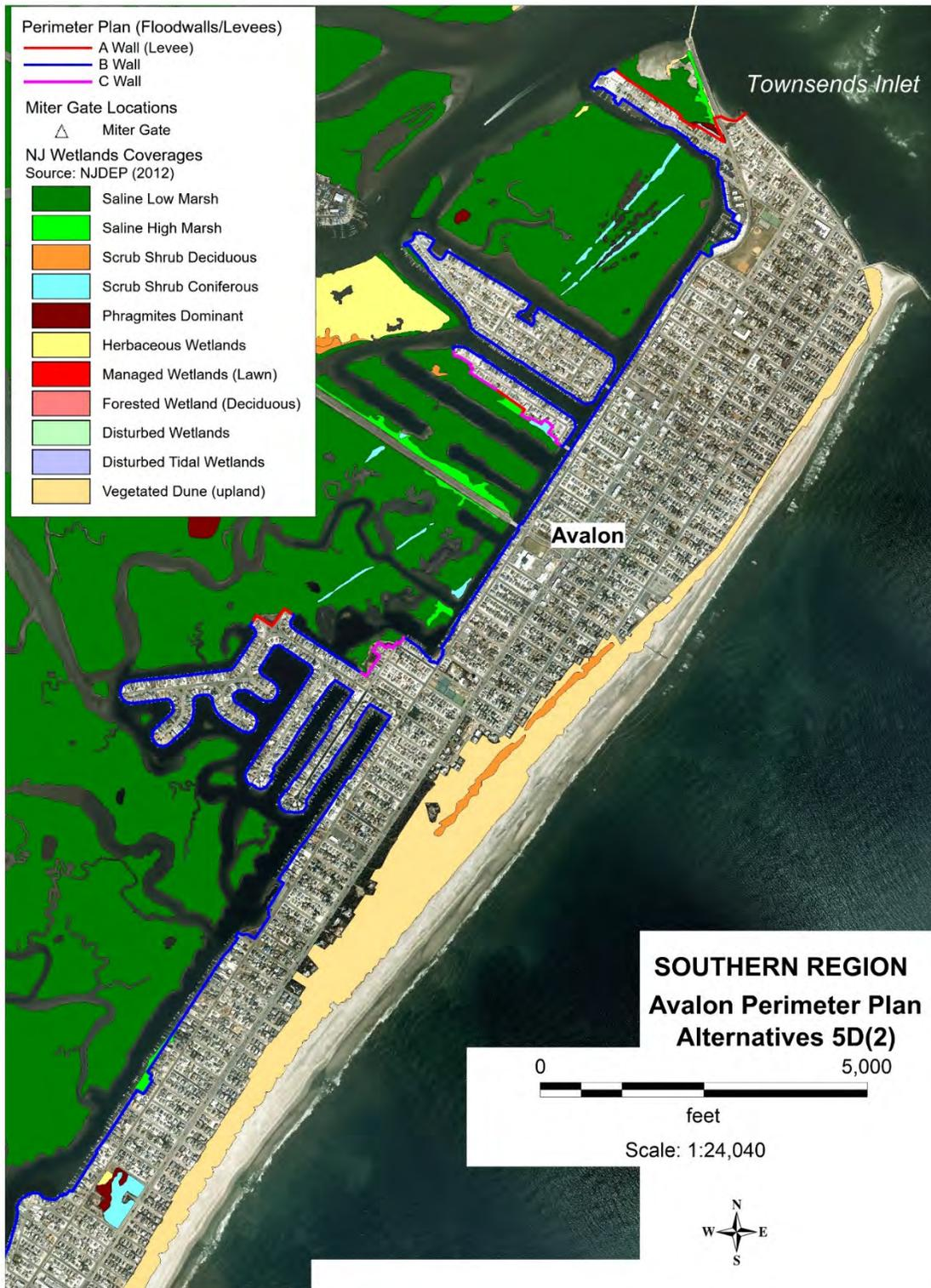
Figure 55: Perimeter Plan Overlay with Wetland Habitats along Avalon Alignment in Alternatives 5D(2)
