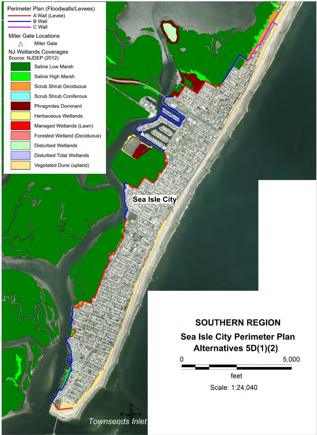
Figure 53: Perimeter Plan Overlay with Wetland Habitats along Sea Isle City Alignment in Alternatives 5D(1) & (2)
